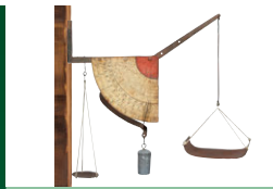
1769 Ancestor Johann Jakob Sauter built the Hahn inclination scale out of iron, a foundation stone for weighing for the balance industry in Southern Germany
